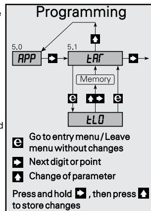
When submenu 5.1 has been selected for {tLO or tHI}, activating the **◀** key for more than 2 s will save the input value to the value it had when activated. The input span is not affected but is kept relative to the new offset value.
